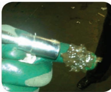
Use magnet to determine if debris In lube is metallic
