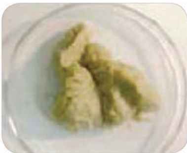
Lube contaminated with water
