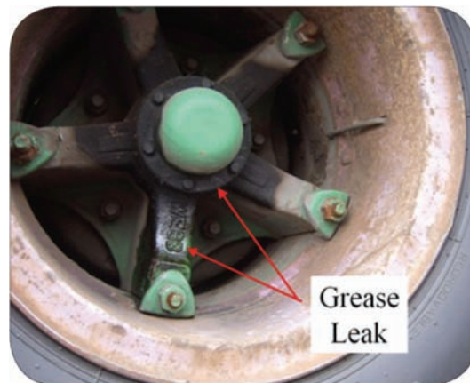
Significant wetness/inspect wheel end
