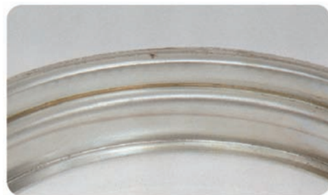
Seal running path also shows angled wear
