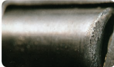
Roller end wear
