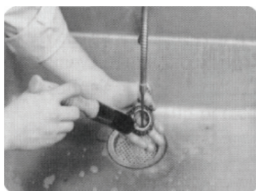
Proper bearing cleaning
