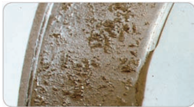
Contaminated lube or improper installation or wear
