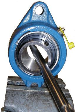
Be sure that the housing and bearing are designed to be used together. SKF uses two small holes on the opposite sides of the outside diameter raceway and 180 degrees apart from one another to line up with a channel machined into the flanged housing unit, as most manufacturers do, to ensure our adapter bearings will be properly lubricated in accommodating housings.
