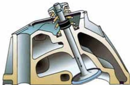
Positive seals attach to the valve guide boss. They work like a squeegee, wiping and metering oil on the stem as it passes through the seal.
