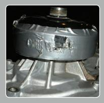
Shown here is the result of an attempt to secure the water pump pulley with a pipe wrench. Despite the use of duct tape, the wrench has damaged the pulley's mating surface, destroying the water pump.
